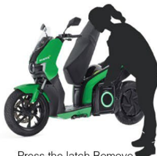
Press the latch Remove the battery pack
