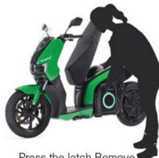
Press the latch Remove the battery pack
